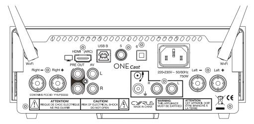
The Cyrus ONE *Cast* is designed in a clean, simple, elegant non-ferrous chassis that minimizes eddy currents and reduces pickup of external noise. Extensive mains supply filtering is used to reduce the impact of this noise which has the ability to colour the audio performance.
